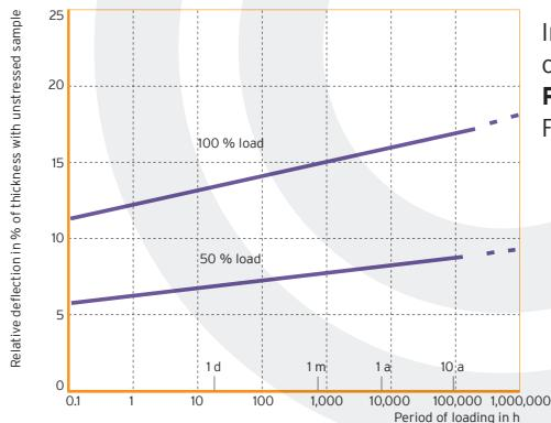
Increase in deformation under consistent loading
