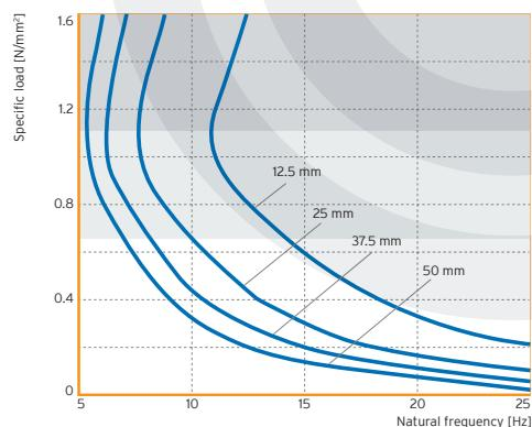
Static modulus of elasticity as a tangent modulus taken from the load deflection curve; dynamic modulus of elasticity due to sinusoidal excitation with a velocity level of 100 dBv re.  $5 \cdot 10^{-8}$  m/s; test according to DIN 53513
