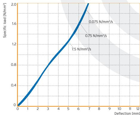
**Dependency on amplitude:** preload at static load limit; Form factor: g=3, thickness of material 25 mm
