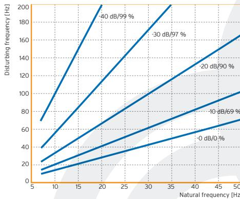
Reduction of the transmitted mechanical vibrations by implementation of an elastic bearing consisting of Sylodyn® NE
