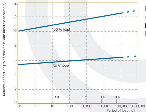
Increase in deformation under consistent loading
