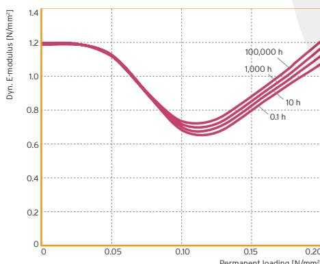
Change of dynamic modulus of elasticity under consistent loading (at 10 Hz)
