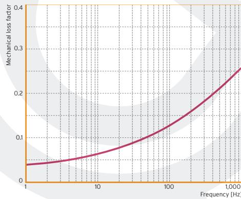
DMA-tests; mastercurve with a reference-temperature of 21 °C; tests within the linear area of the load deflection curve, at low specific loads
