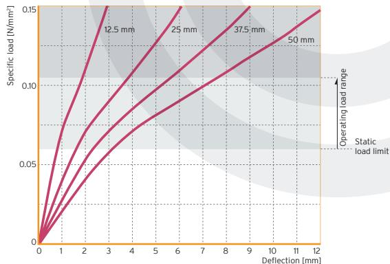
Quasi-static load deflection curve measured at a velocity of deformation of 1% of the thickness per second; testing between flat steel-plates; recording of the 3<sup>rd</sup> loading; testing at room temperature
