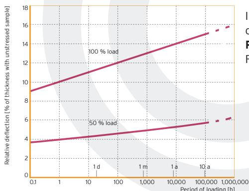
Increase in deformation under consistent loading
