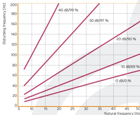
Reduction of the transmitted mechanical vibrations by implementation of an elastic bearing consisting of Sylodyn® NB
