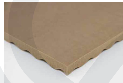
Acoustic Floor Mat 31 Load range: 5000 kg/m 2 Dyn. rigidity s_t' \leq 17 MN/m 3 Improvement of impact sound \Delta L_w \geq 31 dB
