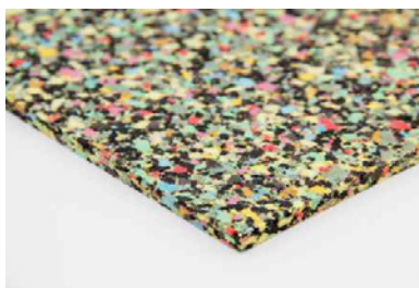
Acoustic Floor Mat 21 Load range: 2500 kg/m 2 Dyn. rigidity s_t' \leq 40 MN/m 3 Improvement of impact sound \Delta L_w \geq 21 dB
