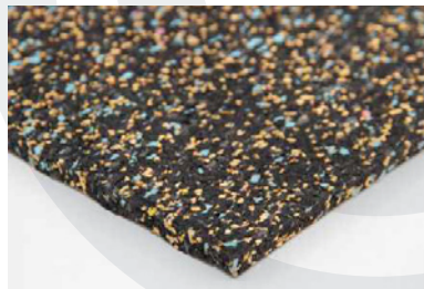
Acoustic Floor Mat 26 Load range: 5000 kg/m 2 Dyn. rigidity s_t' \leq 20 MN/m 3 Improvement of impact sound \Delta L_w \geq 26 dB
